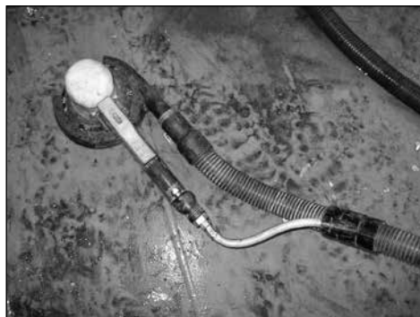
Grinder with a HEPA exhaust attachment
